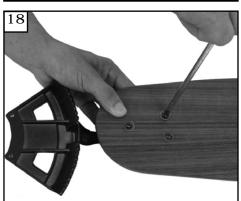
Attach blade arms to blades using the blade arm screws and washers provided.
